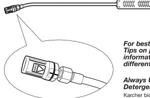
**Step 1** To apply detergents the triple jet nozzle must be set to the "CHEM" position.
